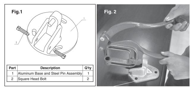
The Mounting Base attaches to a bench top or table (capable of supporting the weight of the Mounting Base and workpieces) using bolts or screws (not provided). The Deep Throat Hand Punch (SKU 91510) slides over the pin in the base as shown in Fig. 2. Secure the Hand Punch by tightening the two screws (2) shown in Fig.1 evenly. Periodically check all hardware for tightness.
